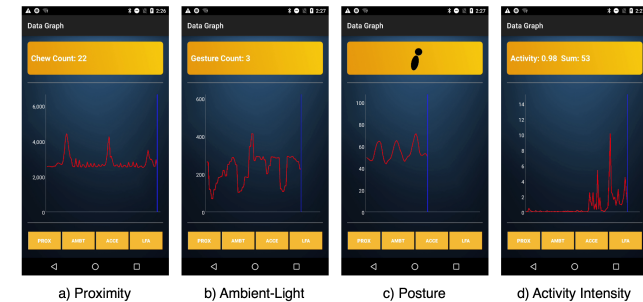
Figure 3: Android app captures four signals and performs real-time calculation of a) chew count, b) feeding gesture count, c) posture, and d) activity intensity estimation.
