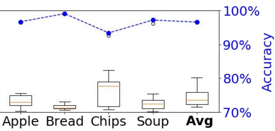
□ We show, given a limited number of known food items provided to a bedridden participant the ability to identify food-type with 97.2% F1-Score, and estimate calories with a 96.6% accuracy using audio, proximity, IMU, and ambient-light sensors around the
