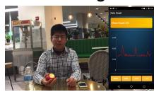
The proximity sensor signal shows 3 bites and 2 chewing sequences between the bites with a chew count of 22.
